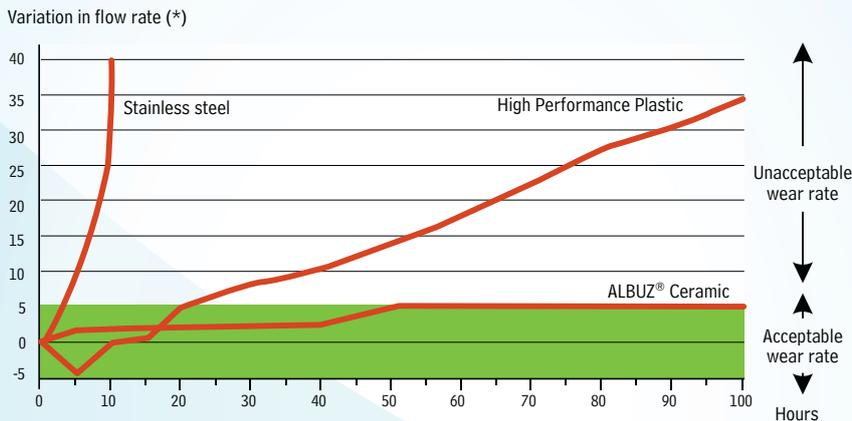
(\*) Flow rate variation due to wear in % - Test in accordance with NFU.26.110 equivalent to ISO 5682-1
